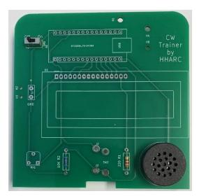
Insert and solder the potentiometer. It has two legs on one side, one leg on the opposite side, and a movable white top. Solder it with the side with the two legs toward the bottom.
