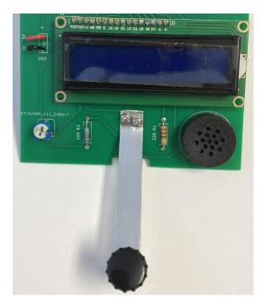
Then take the black nylon spacer and put it through hole 1 (H1) at the top of the PCB. Tighten with its nylon nut.
