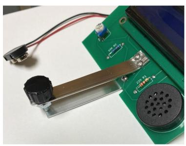
If necessary, adjust the angle of one or both halves of the key so that the bottom half lies flat on the table and the top half has only a small space between the end of the knob's bolt and the bottom half. (No more than 1/8 inch.) IMPORTANT! When manipulating the aluminum strips, be sure to put your fingers on both sides of the bolt; don't just hold the PCB, which may put too much strain on the PCB.
