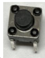
and two button switches
